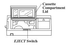
Insert the cassette with the tape window on the left and facing up.
